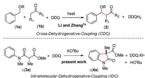
Scheme 1. DDQ-mediated Oxidative C–C Bond Formation
